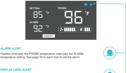
Displays when you lock the controller. The icon will flash if you attempt to adjust the controller while it is still locked. Hold the MODE button to toggle the controller lock.
